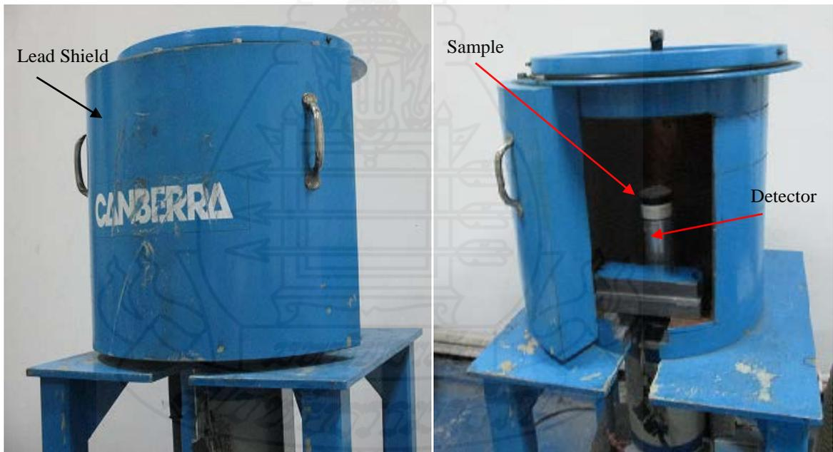
Figure 1: Lead shield to lower gamma background level      Figure 2: Showing HPGe detector inside lead shield
